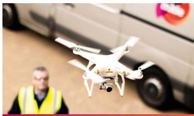
The London Borough of Hammersmith & Fulham (H&F) has welcomed our thermal-imaging drone service to help survey its homes and quickly identify repairs. In place of unsightly and expensive scaffolding, the drones detect problems with buildings faster, resulting in an improved service for H&F tenants, and long-term cost savings for the client.
